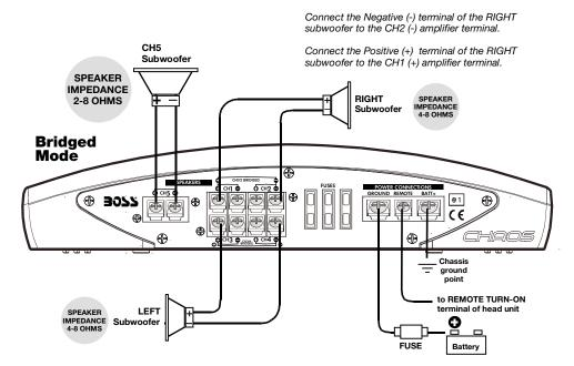
Connect the Negative (-) terminal of the LEFT subwoofer to the CH4 (-) amplifier terminal.
